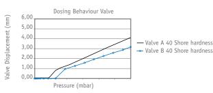
WP developed a proprietary silicone valve solution with a patented technique. The silicone material has a memory for long term seal quality and the opening/closing mechanism. Good temperature resistance is another advantage to give excellent dispensing opportunities for a wide range of viscosities and product applications.
