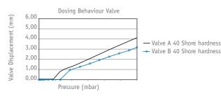
WP developed a proprietary silicone valve solution with a patented technique. The silicone material has a memory for long term seal quality and the opening/closing mechanism. Good temperature resistance is another advantage to give excellent
